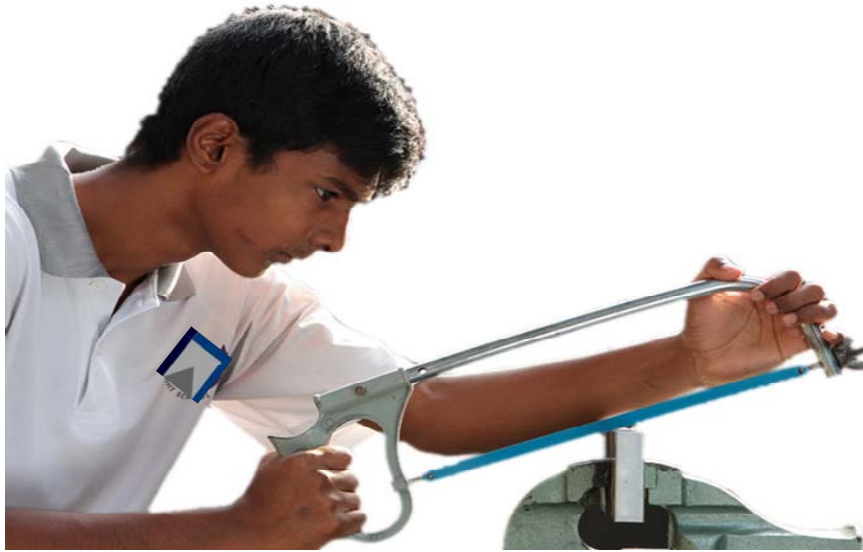
Fig.4.1: The hack sawing process.
