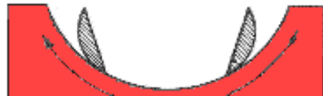
Fig. 5.20: Filing internal curve.
