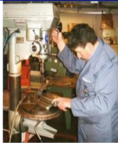
Fig. 6.13: Using the feed handle to lower the drill.
