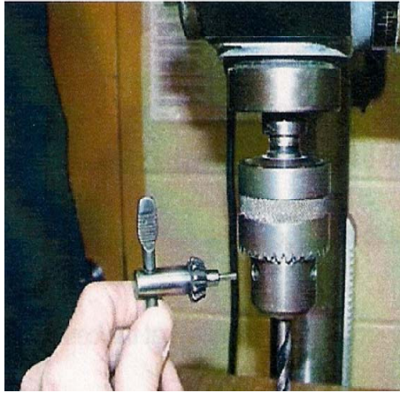
Fig. 6.12: Remove the chuck key after tightening the chuck firmly.
