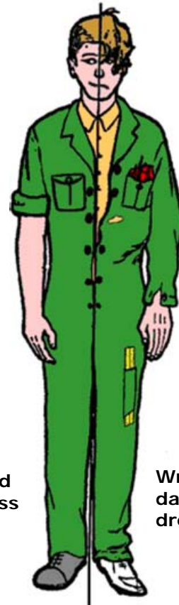
Fig 1.6: Correct and incorrect dress in the workshop
